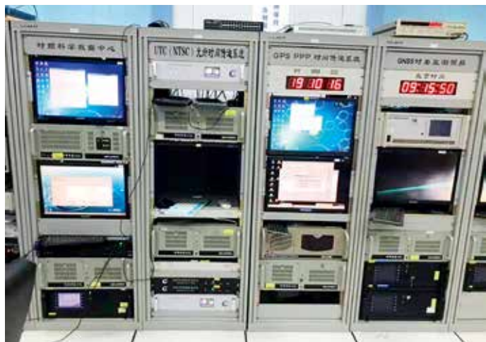
Figure 3-2-18 Optical fiber time transfer device being applied to the time monitoring of the Beidou satellite navigation system
