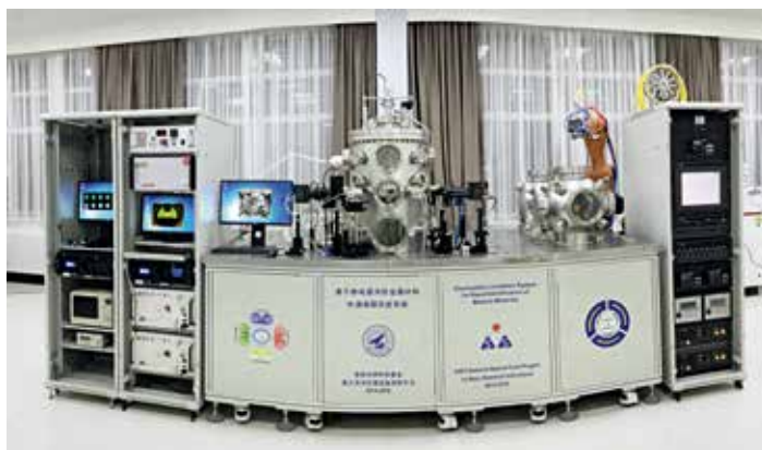
Figure 3-2-9 Electrostatic levitation system for rapid solidification of metallic materials
